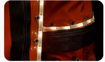
Fot. 4. Widok taśmy z diodami typu LED SMD Photo 4. A view of the tape with LED SMD diodes
